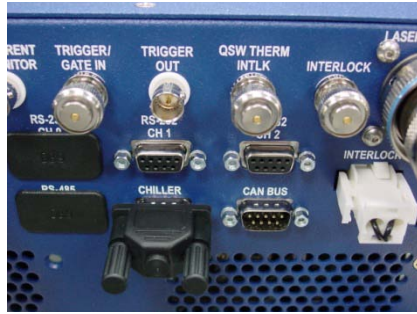
Figure 4-15 BNC Interlock Connection
