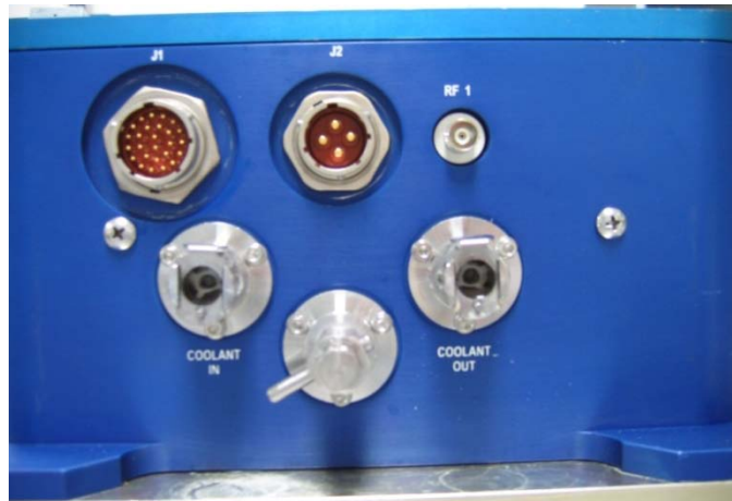
Figure 4-5 Connectors on the rear panel of the Patara-IR TEM 00 laser
