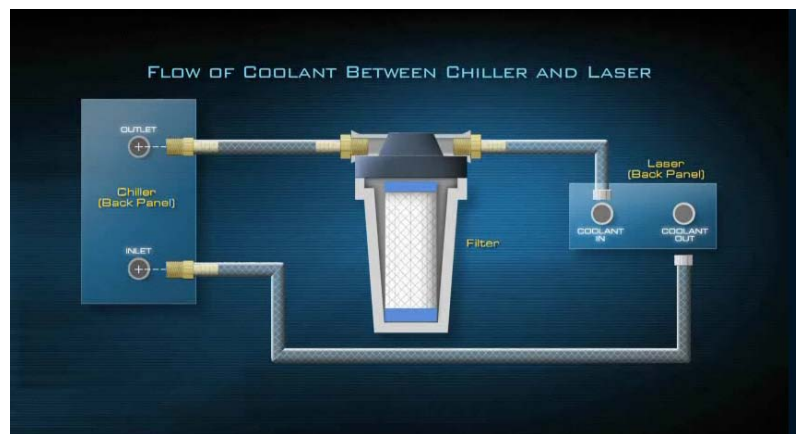
Figure 4-3. Coolant Hoses and Filter Connections
