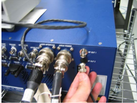
Figure 4-12 RF Signal Cables
